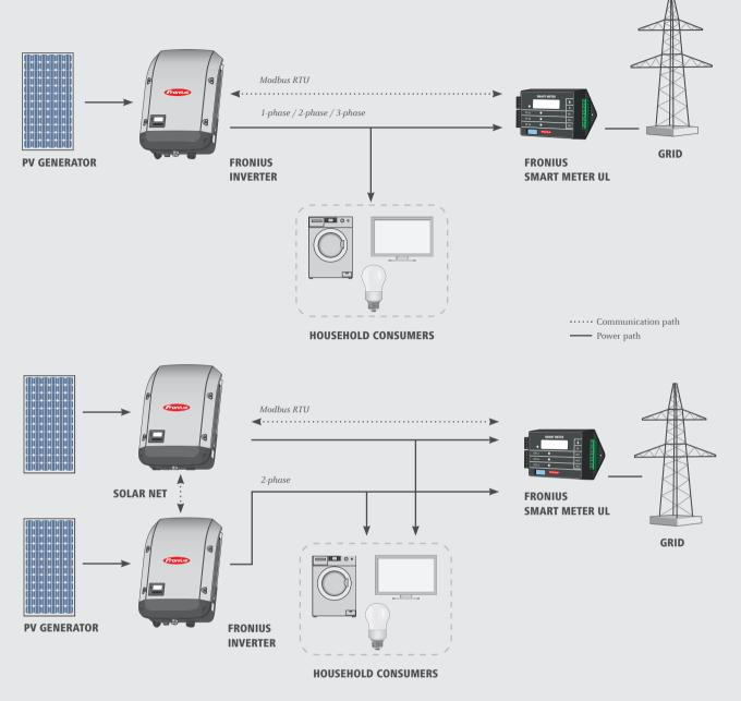
/ The Fronius Smart Meter UL works in conjunction with the Fronius Datamanager 2.0 via the RS485 interface (Modbus RTU) on the Fronius IG Plus inverters. The Fronius Smart Meter UL can be retrofitted at any time together with the Fronius Datamanager 2.0 on all Fronius inverters.
