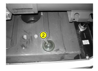
• Do NOT fill the tank over the maximum level by checking it on the specific page of the display of the electronic board for "Automatic panel with standard electronic board" or by inspecting it visually in the case of "Manual panel with digital board".
