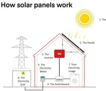
If more power is produced than what is consumed, the excess power will flow back into the grid through the meter. If more power is required than what the Solar PV system can produce, the balance is made up from the grid and is recorded by the meter. (Note: Some systems are limited in their export amounts by the electricity retailer and supply authority, these systems may not feed electricity back into the grid)
